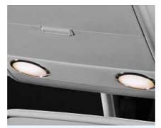
The cab features one interior light and two reading lights in the roof console, while the rear passenger compartment features an additional four interior lights and four reading lights.
